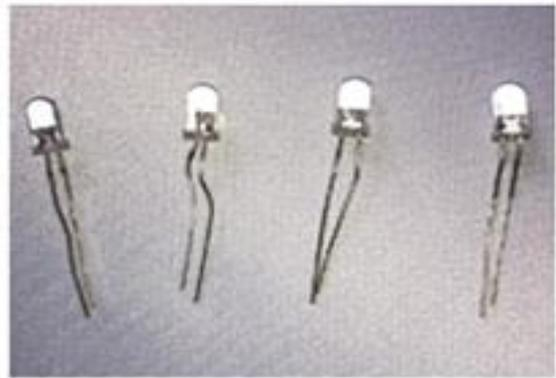
Figura 4 – Quatro LEDs coloridos
