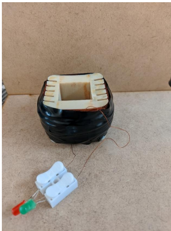
Figura 2. Bobina conectada com os LEDs. (Autor, 2025)
